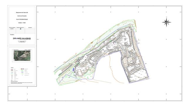
Chuzelles Open quarry (department of Isère), December 2015. Topographic survey conducted from 1436 vertical shots made by the company Infratech and topographic map published by Drones Imaging including:
